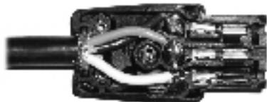
Position the cable so that its black insulation ends just inside the plug. Then run each of the three wires so that it fits under its screw from the left side. It will look like this:
