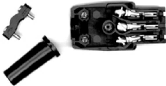
The clamp and tube at left, if they are included (sometimes they are not), can be discarded. Carefully loosen the three screws, but don't remove them completely. The top screw (as seen in this photo) is for the live (brown) wire, the bottom one for the neutral (blue) wire, and the middle one for the ground (green) wire. *Do not under any circumstances interchange them!*
